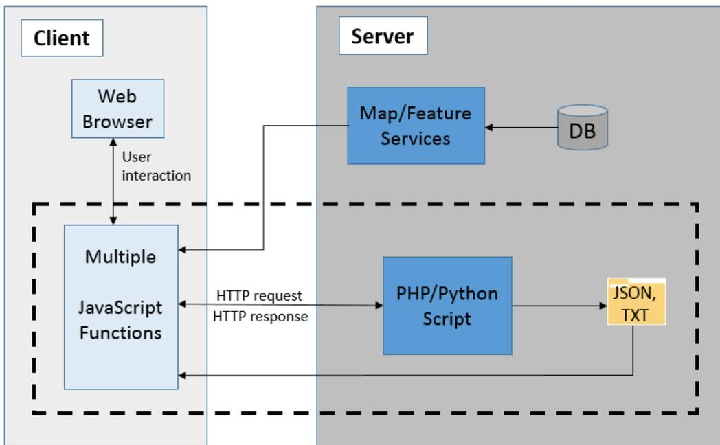
**Figure 1:** MILES online comment architecture overview. The components within the dashed box can be implemented on any web server.
